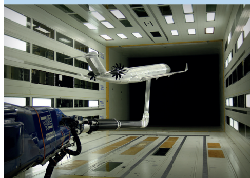
Figure 4 Counter rotating open rotor model (EU CleanSky Z08 project)
