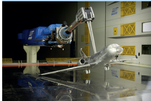
Figure 3 Business jet model in ground effect (EU CleanSky PLAAT project)
